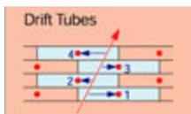
For simplicity, the drawing to the left depicts the drift tubes having a rectangular cross section; however, the actual drift tubes in CMS have a hexagonal cross section
